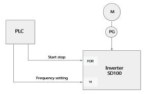
1.PLC supplys start signal and speed signal(0~10v)
