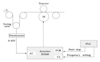
Traction is solely controlled by frequency converter PID (from zero to maximum running frequency)
