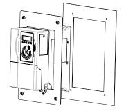
Step 3: Fix the drive in the device hole by four screws.
