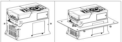
Step 1: Remove the two ground screws, Step 2: Place the flange on the drive front cover, use take the nuts from the accessory kit and the four screws (in accessory kit) to fasten the flange, and install the ground screws.
