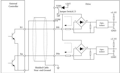
While using this mode, J3 1-2 must be connected (default state: VDD connects to OP).
