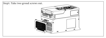
Step2: Both sides use M4 screw locking, and the screw length must not exceed 10mm.
