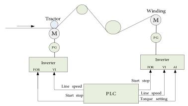
Winding (With speed feedback torque control+Diameter counting +Friction and Inertia compensation)
