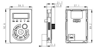
When installing LCP-02 outside, a cradle is needed. The external dimensions of the cradle are shown below (unit: mm):
