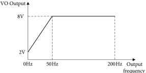
If C06.73 = 80.00% (40Hz), C06.74 = 10.00% (5Hz), then the relationship between the output frequency and VO output is shown below:
