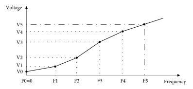
C01.55[0]~C01.55[5] is respective to V0~V5, C01.56[0]~C01.56[5] is respective to F0~F5, Vn is motor rated voltage, Fn is the motor rated frequency.
