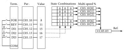
In the preceding figure, FOR, REV are set as two-line mode 1, DI1, DI2 and DI3 are used as the multi-frequency input terminals, each of which has a bit value. The state combinations of these terminals correspond to multiple frequencies, When (DI3, DI2, DI1) = (0, 1, 0), the state combination value is 2, corresponding to the value set in C03.10[2]. The target running frequency is automatically calculated by C03.10[2] x C03.03.
