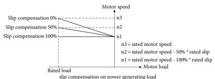
When having more than one motor on the same shaft there is a need for some kind of load share between the drives controlling the motors. This has typically been made with two drives running in speed open loop mode and one with negative slip compensation.
