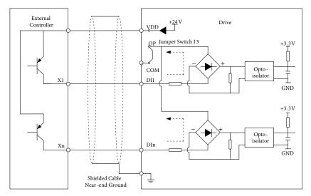
While using this mode, J3 2-3 must be connected (COM connects to OP).
