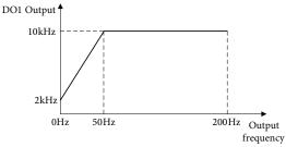
If C05.63 = 80.00% (40Hz), C05.64 = 10.00% (5Hz), then the relationship between the output frequency and DO1 pulse output frequency is shown below:
