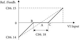
Point A as shown in the figure is the analog value that corresponds to a setpoint that equals 0. It is calculated via analog low, high values and low, high reference/feedback values. After set terminal VI zero dead band, UAB=UAC=C06.18/2. If the VI input is between B and C, the VI reference/ feedback is 0.
